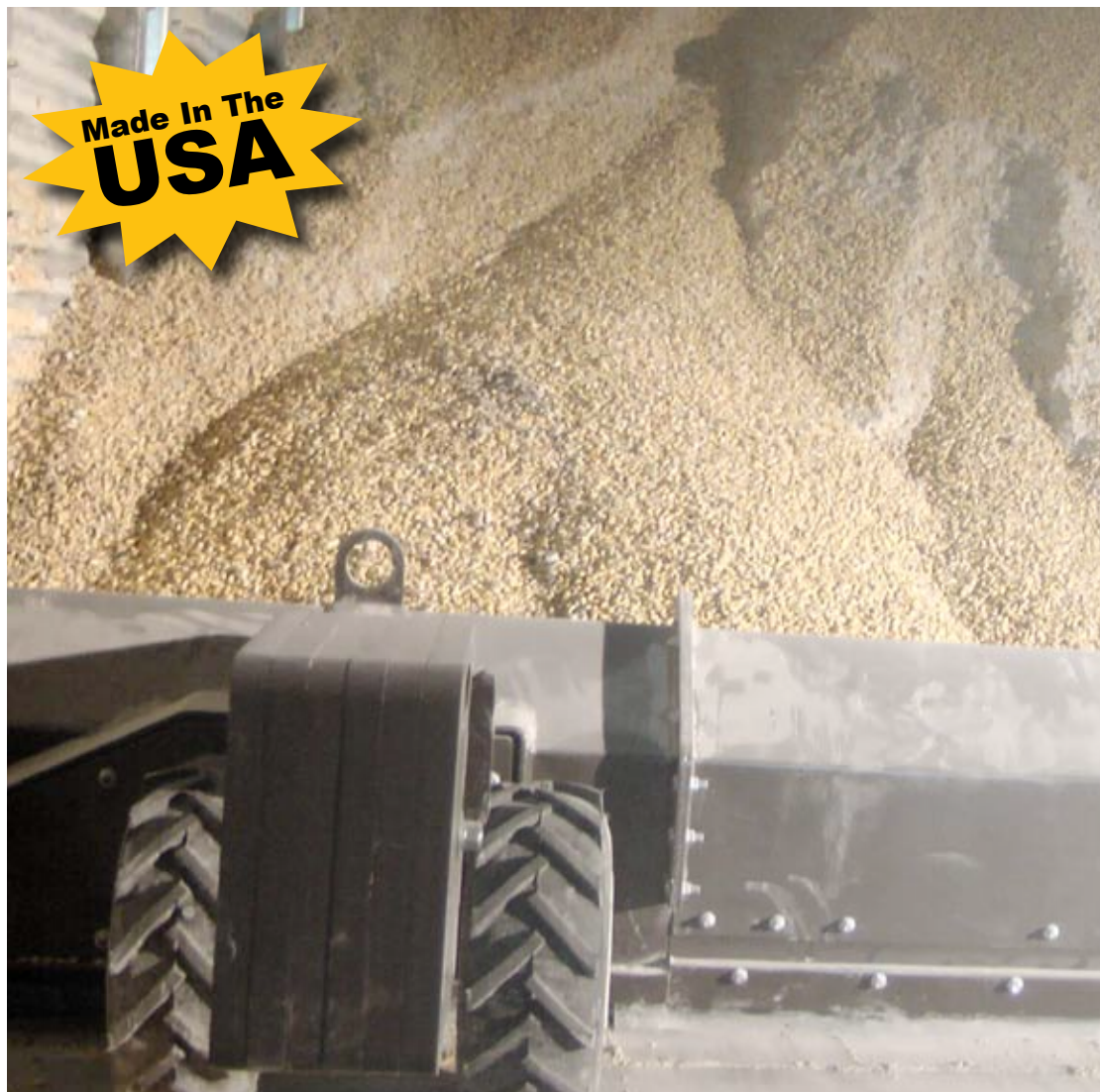
Tires are foam filled, with a tractor tread. Drive tire size is 13 x 5.00-6 Super Lug.
